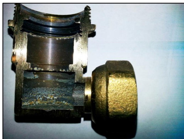
Visible signs of corrosion on un-watermarked brass fitting
